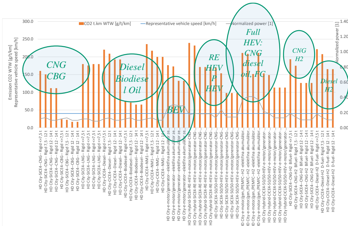
Figure 6: Specific green-house gas emissions for different lay-outs of city heavy duty commercial vehicles with groups from Figure 5
